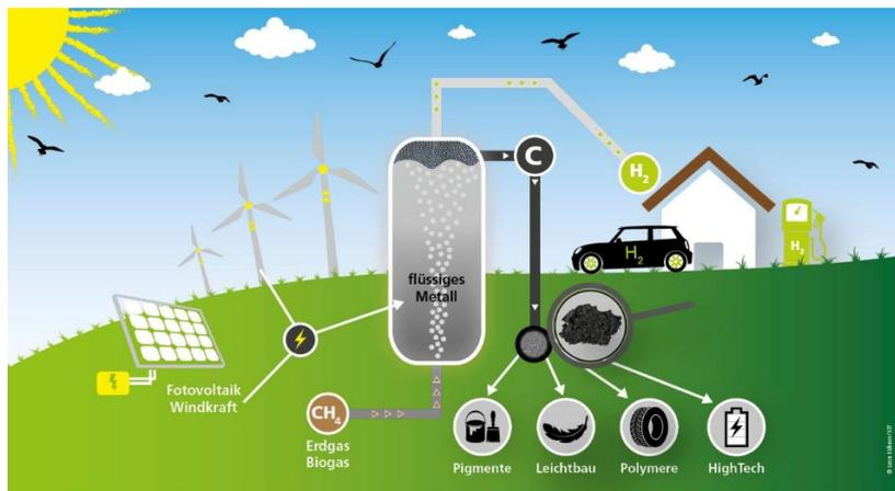
Methane pyrolysis by means of a bubble column reactor allows for the climate-friendly use of fossil natural gas. (Graphics: Leon Kühner, KIT)
