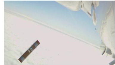
For the first time, the newly developed KITsonde will be used: sensors will be dropped from up to 13 km flight altitude to measure temperature and moisture of the atmosphere. (Photo: DLR)
