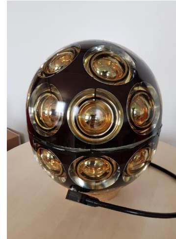
Prototype of one of the new detectors to measure Cherenkov radiation in the IceCube upgrade experiment. (Source: DESY, IceCube Collaboration)
