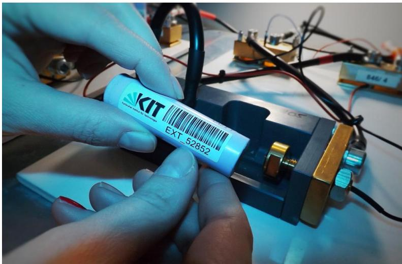
*The quick charging system is based on very long-lived lithium-ion cells and uses a comparably high charging current of up to ten amperes. (Photo: Lea de Biasi/Steffen Jokisch, KIT)*
