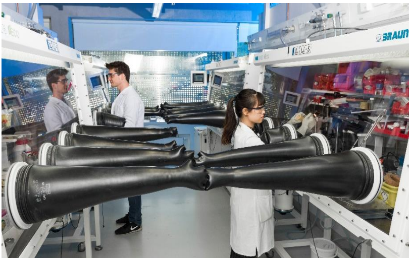
HIU researchers assemble magnesium batteries under organ inert gas atmosphere. (Photo: Laila Tkotz/KIT)
