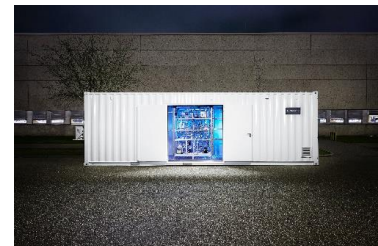
The pre-mounted compact chemical plants fit into a ship container. (Photo: Ineratec/Hauser)
