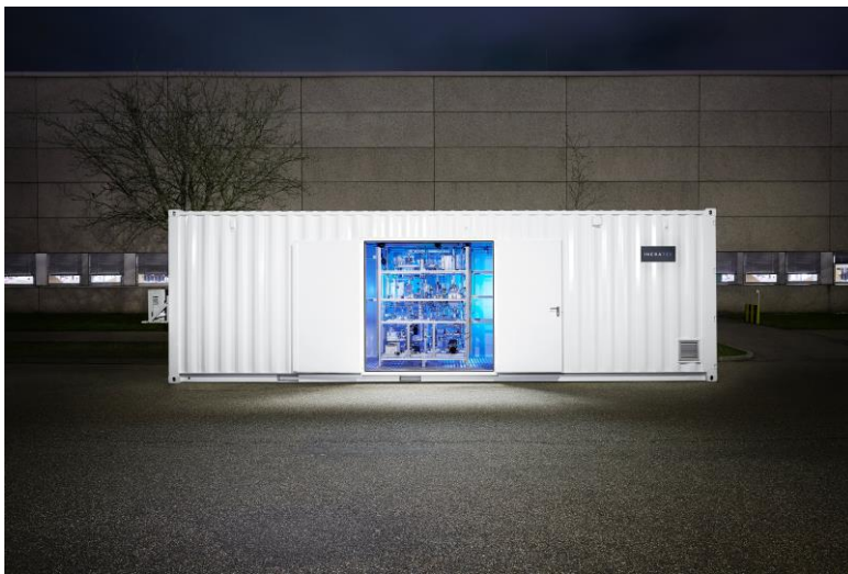
INERATEC builds chemical reactors that are so compact that the entire plant fits into a ship container. (Photo: INERATEC)
