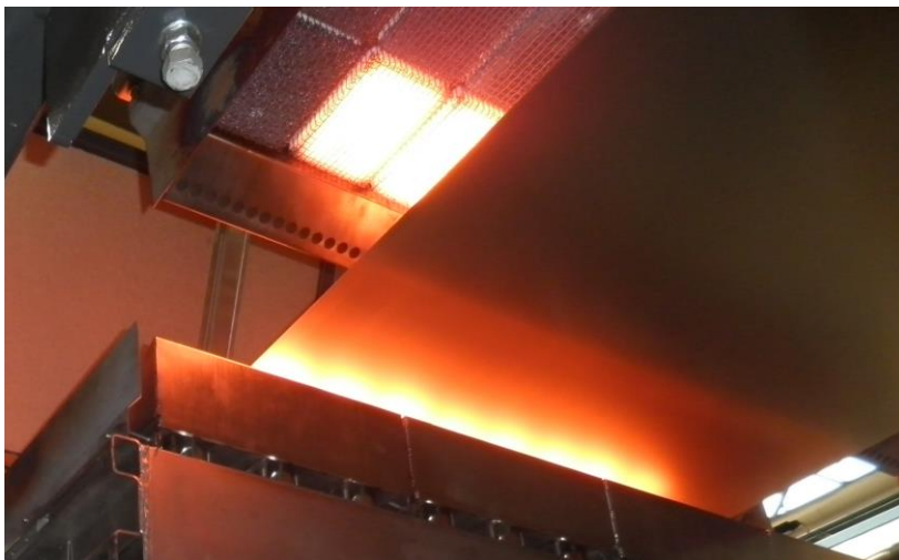
Steel strip drying after pretreatment with an infrared radiant burner (photo: GoGaS Goch GmbH & Co. KG)
