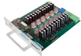
Single-phase voltage source of the modular Power-Hardware-in-the-Loop system (PHiL) for high-performance and highly efficient simulation of the electrical power grid. (Photo: ETI/KIT)
