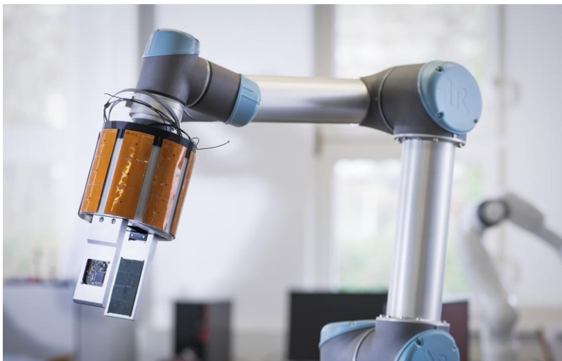
Robot gripper with tactile proximity sensors: Multimodal sensor technology improves collaboration of humans and robots – and enhances safety. (Photo: Amadeus Bramsiepe, KIT)
