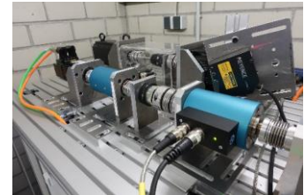
Test rig with integrated power-scaled prototype components according to the sCiL approach. (Photo: IPEK, KIT)
