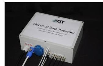
The Electrical Data Recorder supplies high-resolution measurement data from ongoing grid operation – even during voltage losses. (Photo: IAI, KIT)
