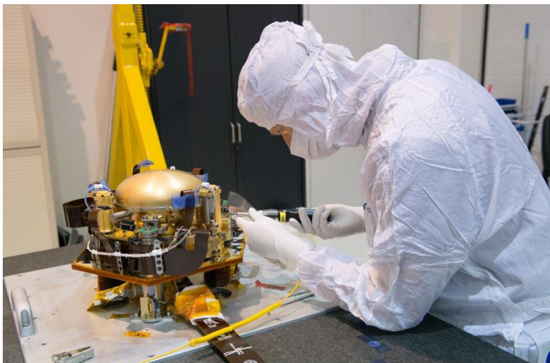
Tests at Schiltach: Seismometer package corresponding to the system that will be used in the "InSight Lander" mission starting in May 2018. (Photo: Copyright CNES)
