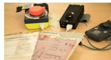
The RescueWave electronic sensor system is to replace slingcards for casualties (foreground). (Photo: FZI Research Center for Information Technology)
