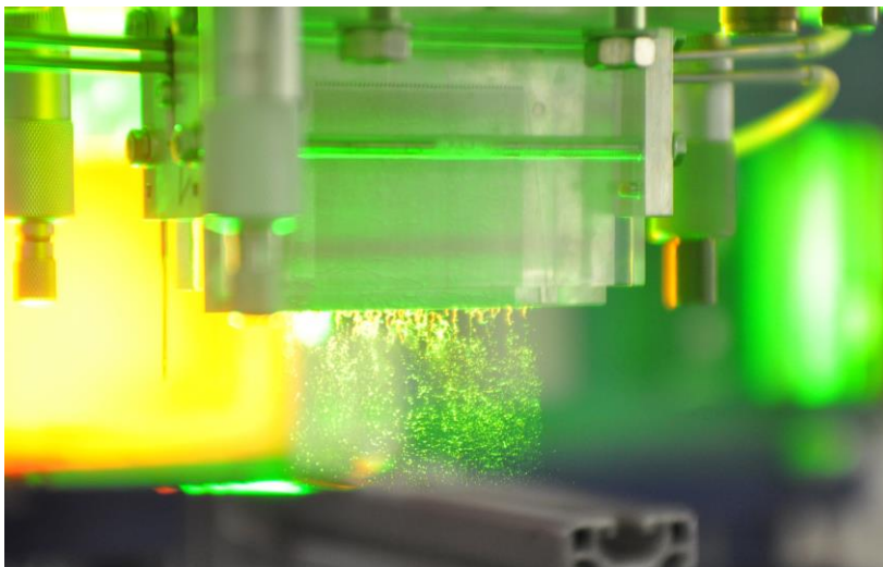
Kerosene atomization experiment: Simulations are aimed at calculating the optimum droplet distribution. (Photo: KIT)
