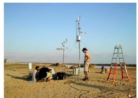
*Energy balance: Stations for radiation and evaporation measurement. (Photo: Ulrich Corsmeier)*
