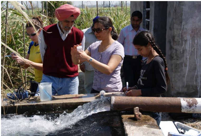
Water sampling with Indian researchers to determine concentrations of selenium and arsenic among others. (Photo: IMG)
