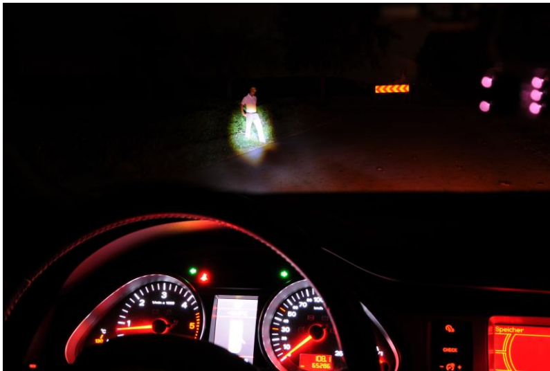
Shedding light into darkness: Driver assistance system light marks persons and deer and, thus, helps prevent accidents. (Photo: Marko H. Hörter, KIT)
