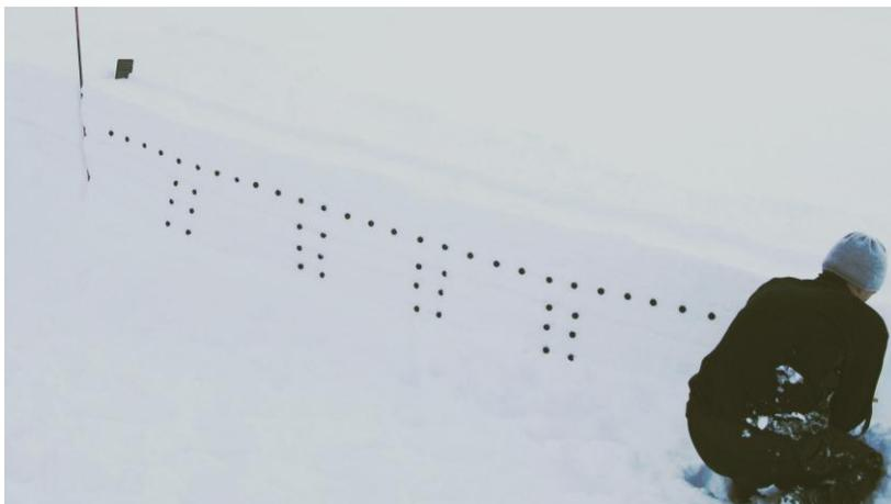
*Development of an avalanche in the snow block: Acceleration sensors in the snow blanket measure breaking speed. (Photo: A. van Herwijnen)*
