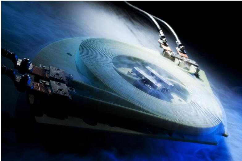
Superconducting coils are cooled with liquid nitrogen and have zero resistance to current flow. (Photo: Martin Lober, KIT)
