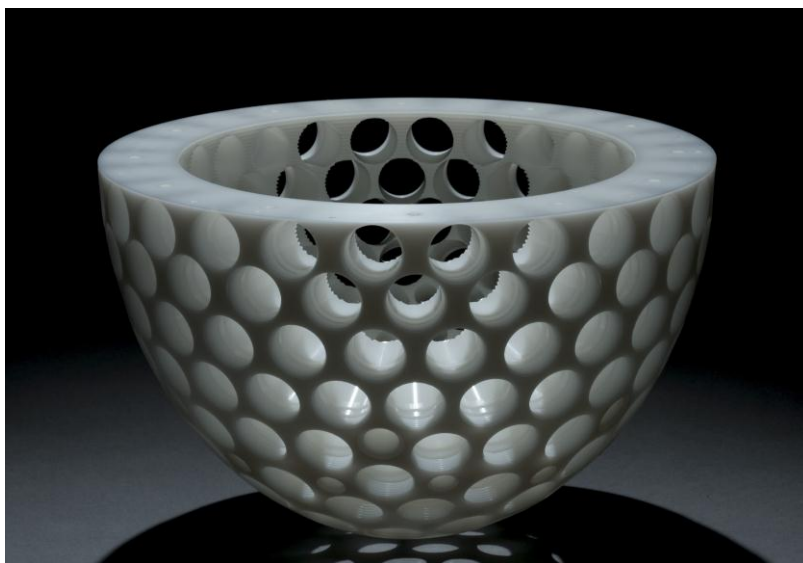
Optimized holder of ultrasonic sensors recording three-dimensional images of the breast. (Photo: Markus Breig, KIT)
