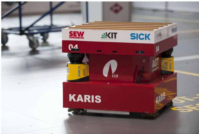
KARIS – autonomous elements optimize materials flow at stores and production halls. (Photo: KIT)
