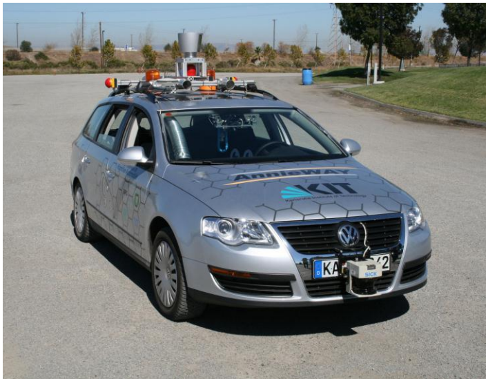
Equipped with sensors and computers, AnnieWAY autonomously finds its way in road traffic. (Photo: Institut für Mess- und Regelungstechnik, KIT)
