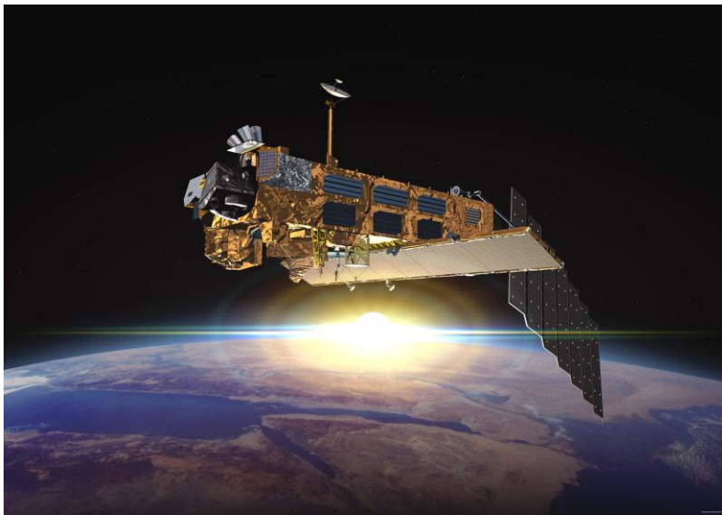
The MIPAS instrument on the European ENVIRONMENTAL SATellite (ENVISAT) measures more than 30 trace gases at the same time. (Picture/Figure: ESA)
