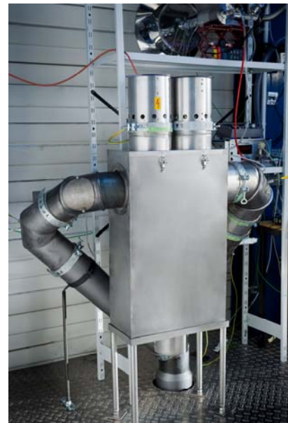
A soot separator for small combustion systems was developed at Karlsruhe Institute of Technology. (Photo: KIT)
