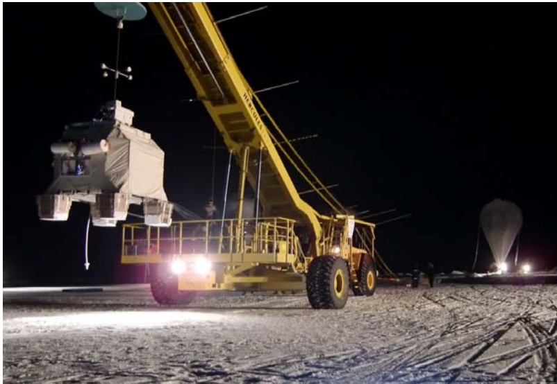
Balloon launch into polar night: In the foreground, the gondola with the scientific experiments. In the background, the main balloon that carries the gondola to a height of more than 30 km. (Photo: Karlsruhe Institute of Technology)
