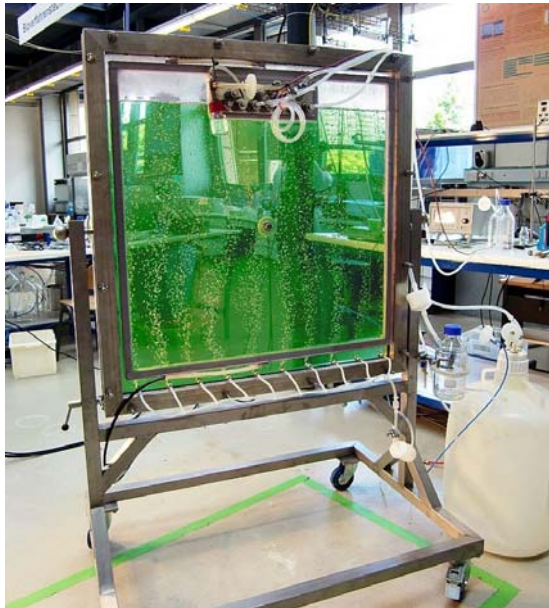
The plate-type reactor at the laboratory ensures optimum light management in the cultivation of algae. (Photo by: Florian Lehr)
