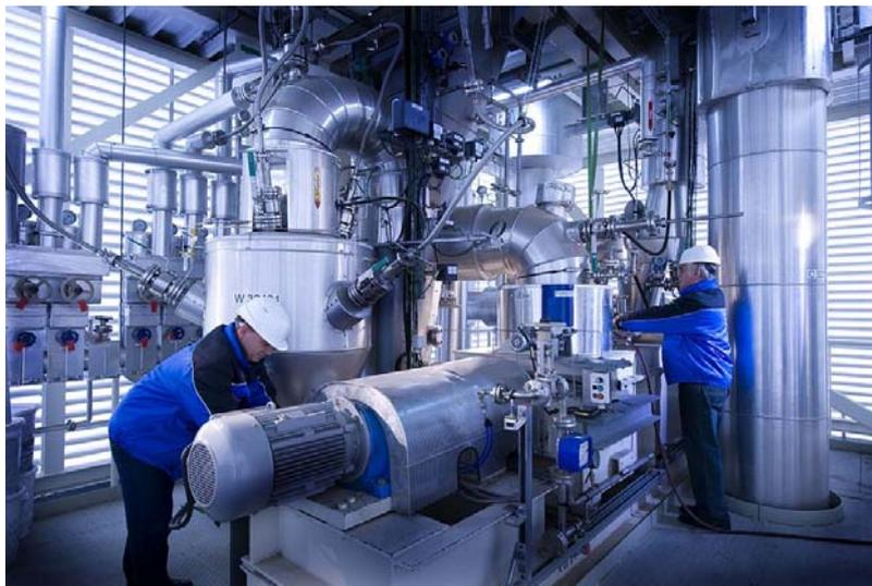
*The reactor producing bioliqSynCrude<sup>®</sup> on KIT Campus North – the first stage of the bioliq<sup>®</sup> process. (Photo by: Markus Breig)*
