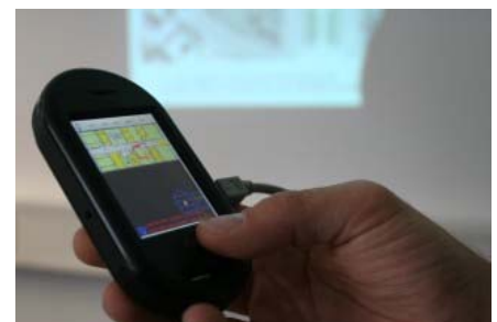
A portable interface shows the map of a building with exact position data. (Photo: Gabi Zachmann)
