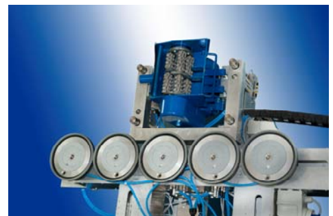
Detailed view of AMANDA with mill and suction plates. (Photo by: Markus Breig)
