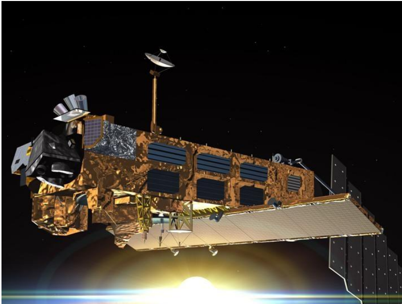
The MIPAS infrared spectrometer on board of the Envisat European environmental satellite (upper left edge) (Photo by: ESA)
