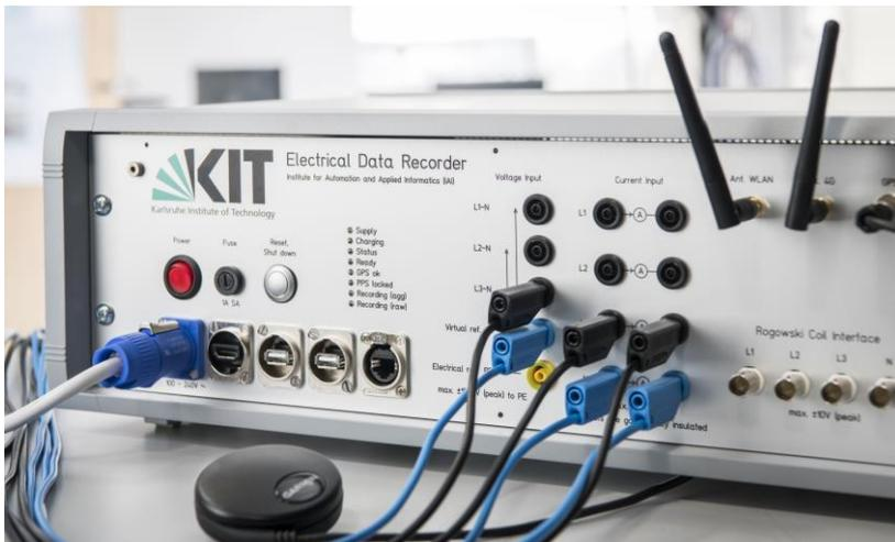
The KIT-developed data recorder uses a GPS receiver and records raw and frequency data with very high resolution. (Photo: Amadeus Bramsiepe, KIT)
