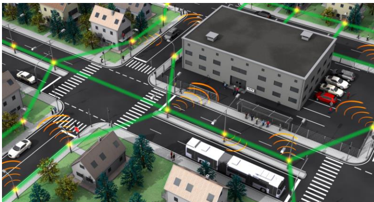
Future mobile network: Small radio cells (orange) are connected by wireless high-speed terahertz links (green). (Figure: IPQ, KIT / Nature Photonics)
