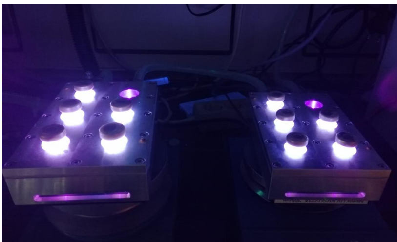
DNA is exposed to UV radiation from LEDs to study how far the photoenergy migrates. (Photo: Arthur Kuhlmann, KIT)
