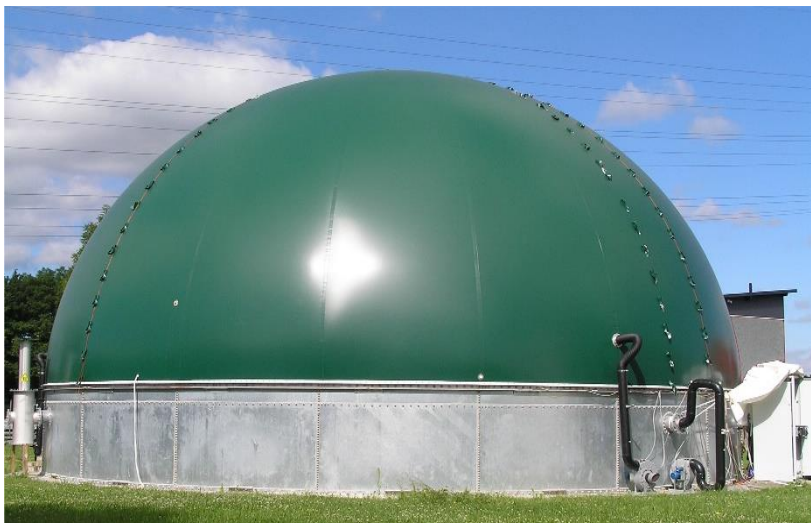
Using a test tank, KIT scientists studied the effects of environmental conditions on fabric membrane gas holders. (Photo: Rosemarie Wagner, KIT)
