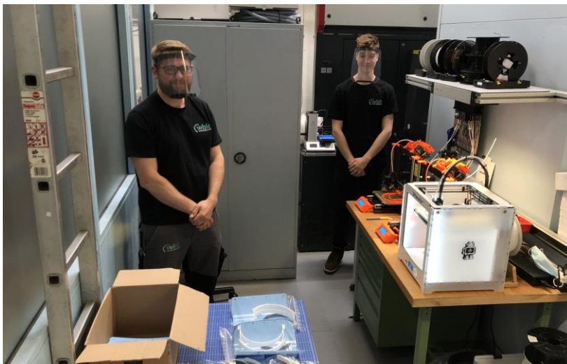
Production of one face shield by 3D printing takes about three hours. (Photo: wbk, KIT)
