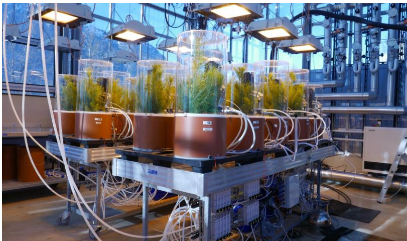
Experimental setup: In high-tech plant chambers, Aleppo pines were exposed to increasing temperatures. (Photo: Plant Ecophysiology Lab, KIT)
