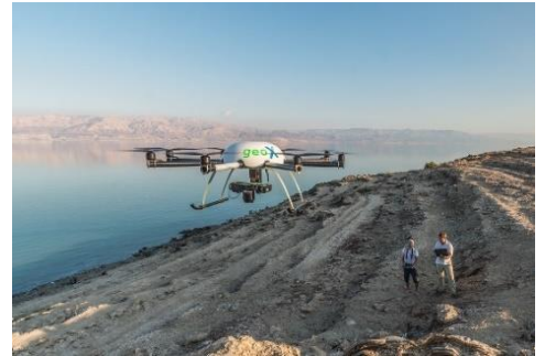
Octocopters produce aerial and thermal photographs of excellent three-dimensional resolution. Scientists use them for digital terrain models to identify underground feeders of groundwater. (Photo: André Kuenzelmann, UFZ)
