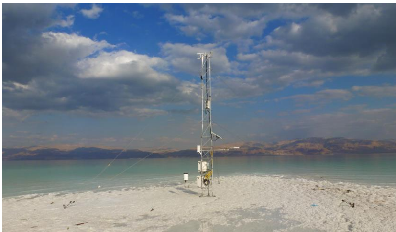
The world's lowest meteorological station located at 429 m below sea level continuously measures evaporation of water of the Dead Sea. (Photo: U. Corsmeier, KIT)
