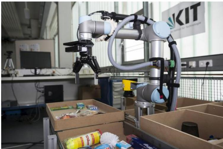
*The IFL PiRo robot detects the objects desired and automatically puts them into shopping baskets. (Photo: Laila Tkotz, KIT)*
