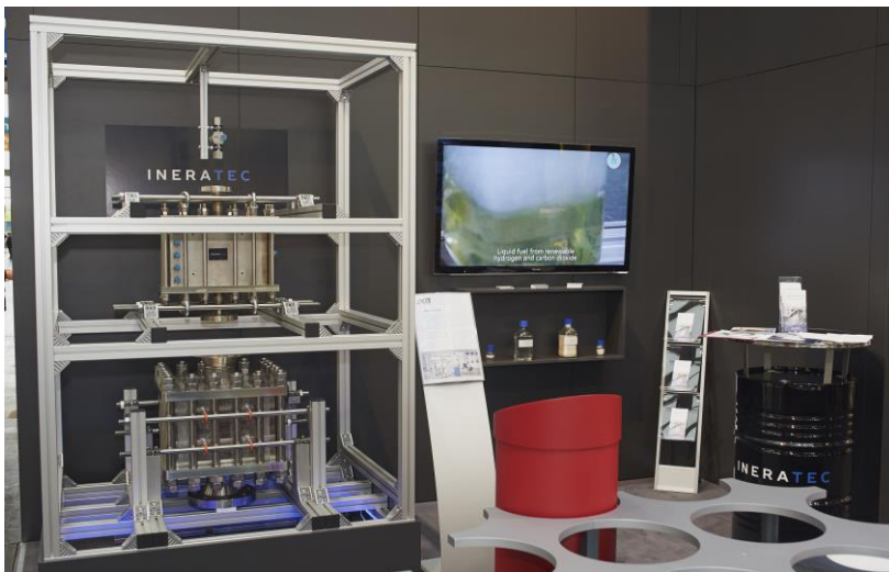
The microstructured Fischer-Tropsch reactor developed by INERATEC, that turns gases into liquid synthetic fuels, was presented at the Hanover Fair 2017 (Photo: Andreas Drollinger/KIT)
