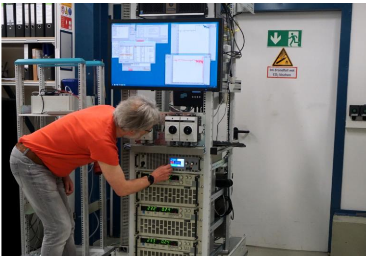
Measuring the efficiency of a storage system. (Photo: KIT)
