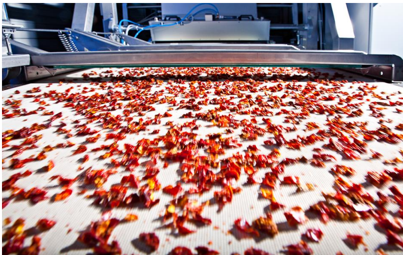
Dried fruit, gravel or waste – all this is sorted on belt systems by size and quality. (Photo: Fraunhofer IOSB)
