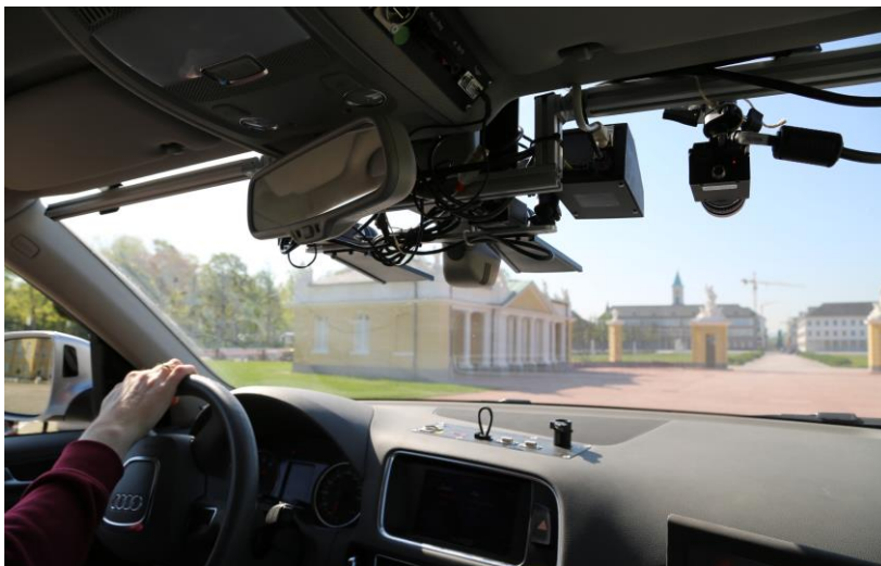
For cars to drive alone through Karlsruhe in the future, route data have to be collected during test drives. (Photo: FZI)
