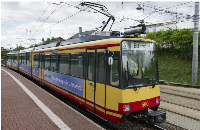
The tram with the instruments on top of the driver's cabin and the AERO-TRAM logo made a total of 6228 measurement drives. (Photo: Patrick Langer, KIT)
