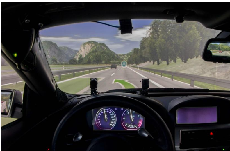
Is the driver ready to take over the steering wheel? Cameras help autonomous systems react to the situation in the vehicle interior. (Photo: PAKoS)
