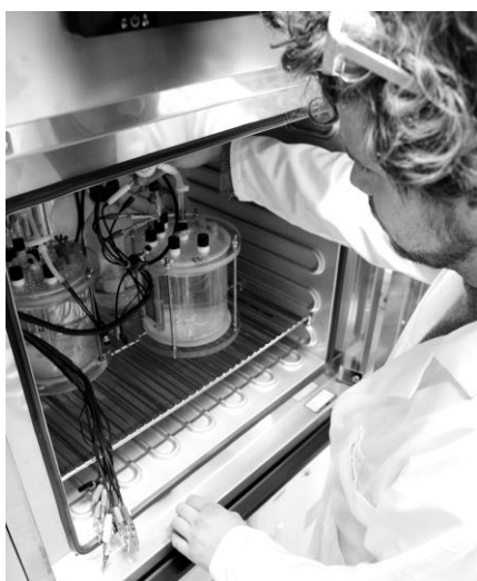
Biologist Johannes Eberhard Reiner, KIT, with the reactors for microbial electro-synthesis. (Photo: Constanze Zacharias)
