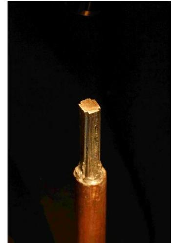
*The inner conductor of CroCo consists of flat, superconducting tapes of different widths. (Photo: KIT)*
