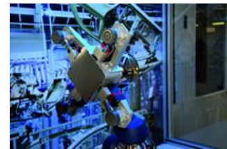
Intelligent gripping system for handling semi-finished textile parts. (Photo: wbk, KIT)
