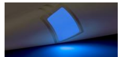
Flexible and curved surfaces can be made luminescent, no matter whether they are made of paper or plastics. (Photo: S. Walter, Binder Gruppe)
