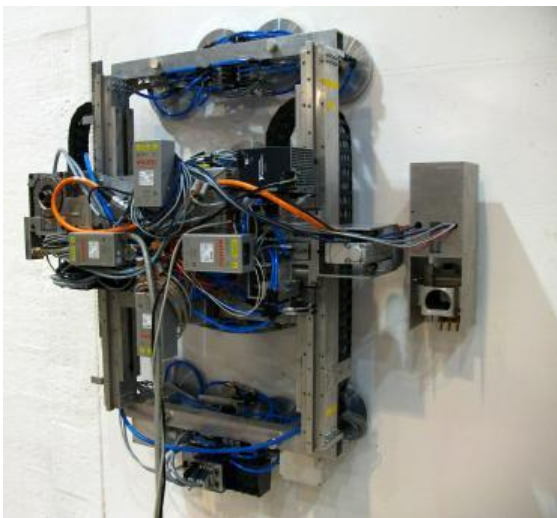
Robots autonomously measure radioactive contamination and decontaminate surfaces in nuclear power plants. (Photo: KIT)
