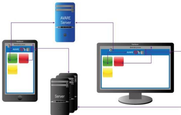
*Functioning of the AVARE System: AVARE encapsulates the application and controls its interaction with the environment. An AVARE server distributes settings. (Source: FZI)*
