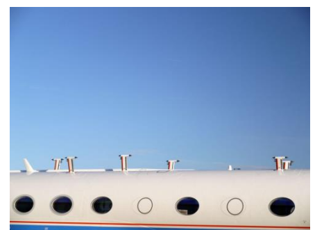
Via seven trace gas inlets atmospheric air is drawn in and directed to the onboard in-situ instruments on board. (Photo: Hermann Oelhaf, KIT)
