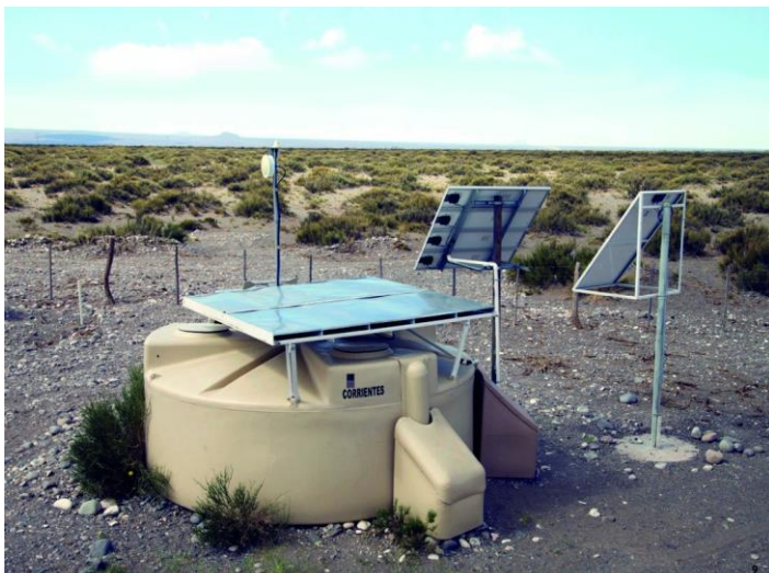
A prototype station of AugerPrime: Every water-Cherenkov detector containing 12,000 l of water is extended by a four-square-meter scintillation detector. (Photo: Pierre Auger Collaboration)
