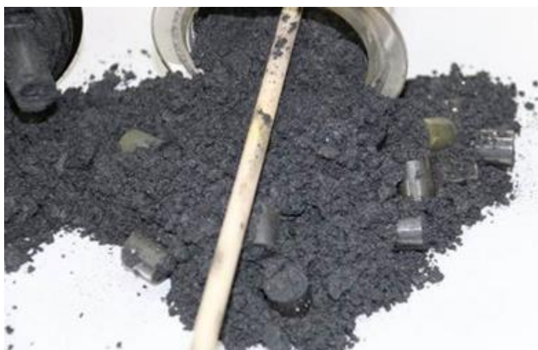
Solid black carbon is a by-product of methane cracking. (Bild: KIT)
